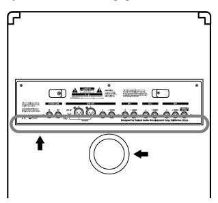
Wrap the AC cord around the cord hook when transporting or storing the unit.
